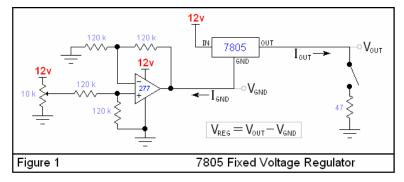
the 10k potentiometer. As  $V_{GND}$  increases,  $V_{OUT}$  should increase at an equal rate.
