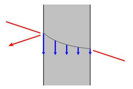
As stated previously, the function of a shield is largely based on the behavior of a wave when it encounters a boundary between two medium. Physical laws explain that the amount of energy reflected depends on the magnitude of difference between the two medium. With regards to electromagnetic waves, reflected energy is determined by the
